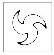
This follows the isoline closely, but results in a shape with varying width - suppose we wanted a shape with constant width instead. We need an estimate of the *closest* distance from a particular point (pixel) to the isoline - if the black/white limit is applied to such a distance estimate, we will obtain a line of reasonably constant width.
